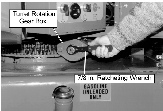
Figure 2-5: Manual Turret Rotation
